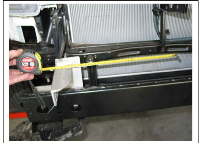
Figure 4 – Drivers side shown centralising steel mounting bracket
