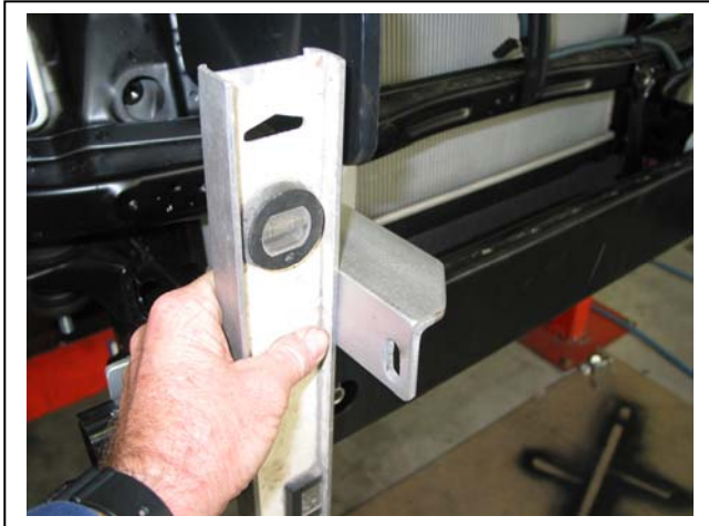
Figure 3 – Shown levelling drivers side steel mounting bracket
