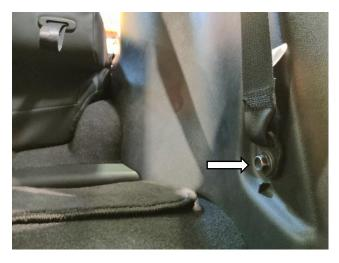
18. Remove (& retain) the indicated fastener from the 3<sup>rd</sup> row lower seat belt mount.
