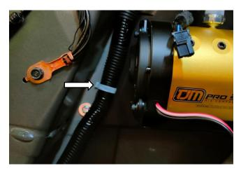
29. Secure the OE electrical harness to the Air Compressor Bracket using the retained cable tie mount as shown.
