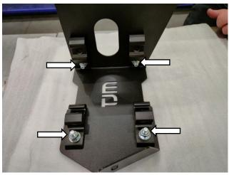
Loosely secure the Mounting Feet (4) on the supplied Air Tank Bracket using M8 x 1.25 x 25mm Hex Head Screws (4), Flat Washers M8 (8) and M8 x 1.25 Nyloc Nuts (4) as indicated.
