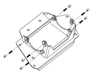
9. Secure Rubber Isolation Mounts (6) & Brass Crush Tubes (6) retained in step 6 on the Air Compressor Bracket as shown.
