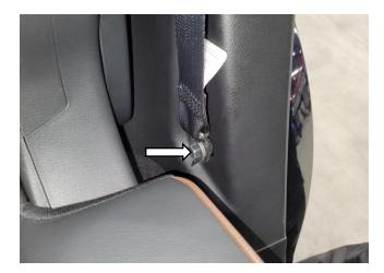
19. Open the passenger side rear door and remove (& retain) the indicated fastener from the 2nd row lower seat belt mount.
