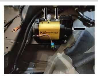
**Note:** It is recommended to install the required air fittings and hose prior to securing the Air Compressor Bracket to the vehicle.
