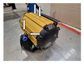
3. Insert the Tank in the Air Tank Bracket by sliding it through the loosely secured Mounting Feet.
