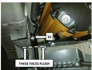
32. Secure Air Tank Bracket using M6 x 1.0 x 20mm Hex Head Screw, 1/4 x Ø3/4 Flat Washer and M6 x 1.0 Flange Nut at indicated location.
