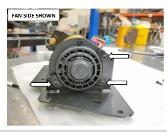
11. Repeat previous step on the fan side of the Compressor to fully secure it to the Air Compressor Bracket.
