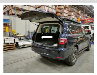
12. Open the luggage compartment of the vehicle and clear the indicated space for Air Tank and Compressor installation.
