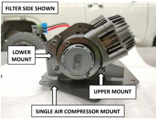
10. Secure the Compressor to the Air Compressor Bracket using the Compressor Mount Plates (Lower & Upper) and the retained fasteners (3) from step 6.
