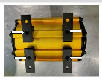
1. Loosen the indicated fasteners (4) to separate the Air Tank from the Mounting Feet (4).
