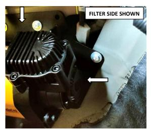
**Note:** The upper and filter side of the Air Compressor Bracket will be positioned in front of the body panels as shown.
