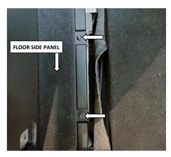
16. Remove (& retain) the indicated fasteners (2) and unclip the floor side panel.
