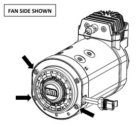
7. Remove (& discard) indicated fasteners (3) from the fan side of the Compressor.
