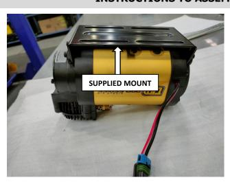
6. Remove (& discard) the supplied Compressor Mounting Brackets. Retain only the fasteners (6), Rubber Isolation Mounts (6), and Brass Crush Tubes (6).
