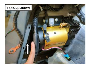
**Note:** Ensure the fan side of the Air Compressor Bracket is positioned behind the body panels as shown.
