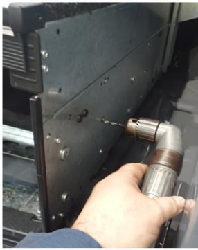
Pilot drilling of marked hole locations
